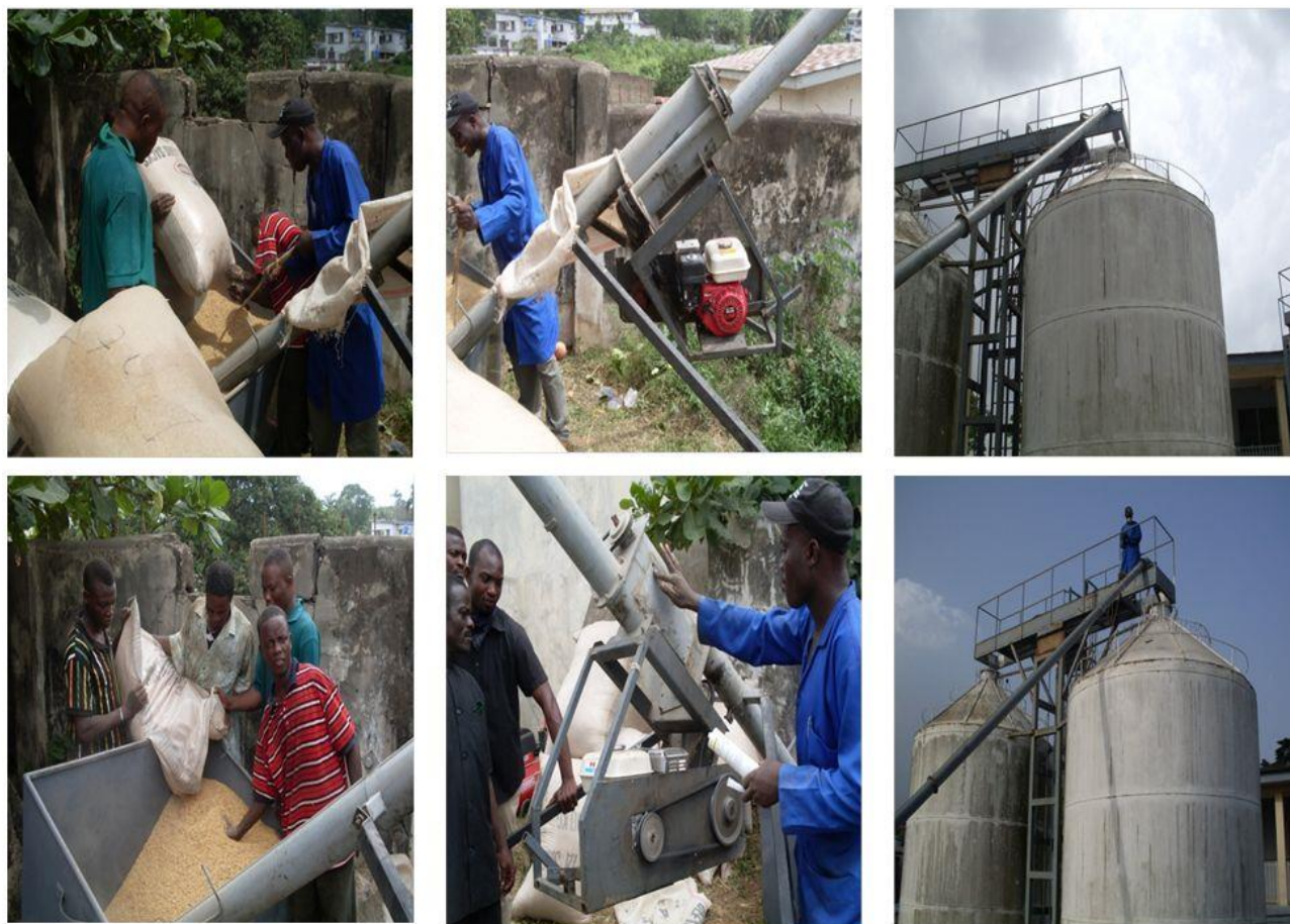
Figure 2. Mechanical loading of paddy rice into a 45 Tones capacity Inert-Atmosphere-Metal-Silo at NSPRI Ibadan in April 2010. a NSPRI = Nigerian Stored Products Research Institute.
